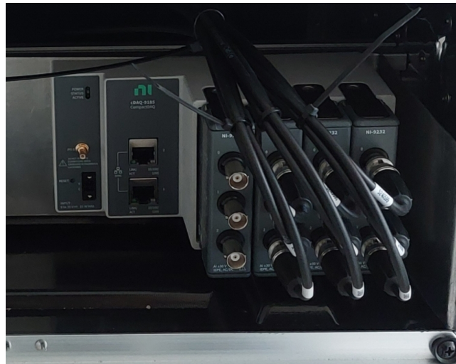
Figure 1.3: Data logging unit based on NI 9232 devices, with high sampling rate.
