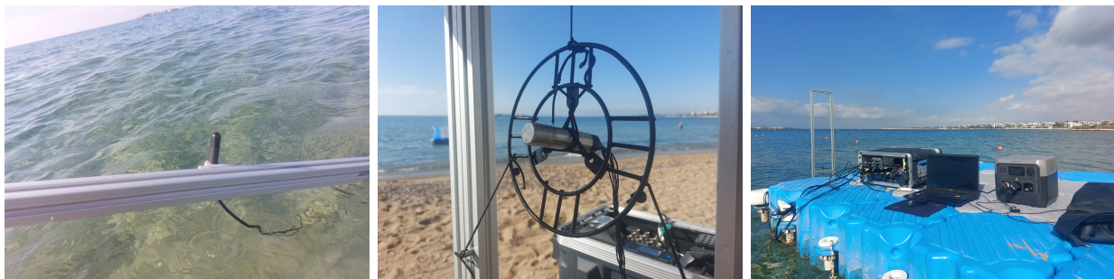
Figure 1.6: INFILI field engineering activities during open-water testing, showing the full acquisition stack deployed on a floating platform alongside vector-sensor and hydrophone evaluation setups.
