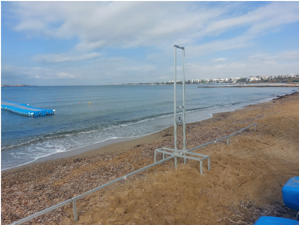
Figure 1.4: Seabed deployment frame for the hydrophone array during coastal field trials.
